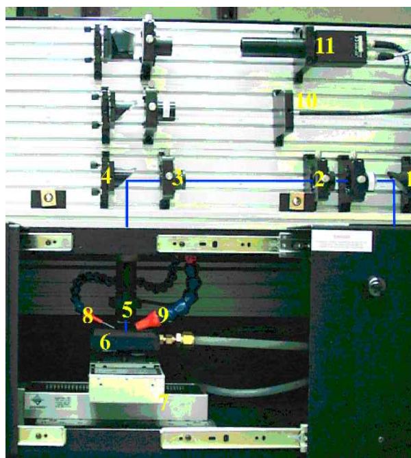
Figure 1. The laser ablation micromachining system. The black line denotes the path of laser emission. The beam is deflected by turning mirror (1) onto aperture (2), passes through iris (3), and is steered by dichroic (4) through the focusing objective (5). The vacuum chuck (6) is mounted on a computer controlled x-y stage (7). The surface of the substrate may be exposed to various gases via nozzle (8) and the vacuum port (9) assists in removal of large debris. The entire process is illuminated with a light source (10) and imaged with a camera (11).
